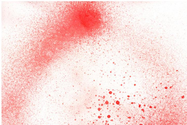
Without **Natural Wet** the spray pattern and droplets are non-uniform and spread apart.
