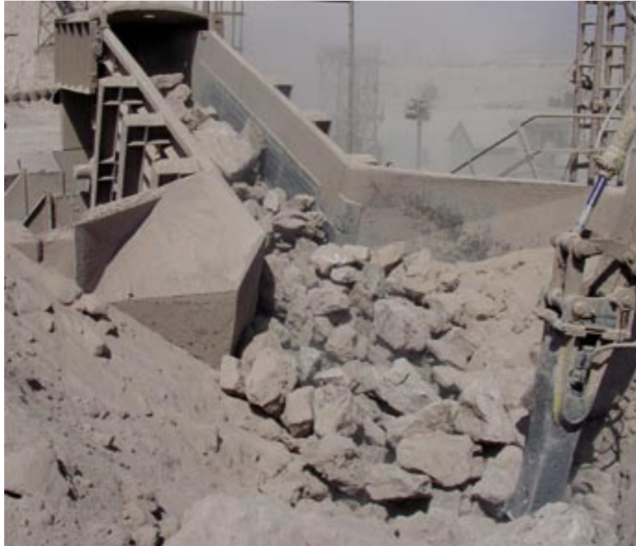
Figure 21: Crushing of the caliche rock before nitrate extraction
