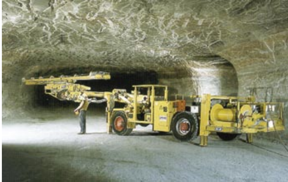
Figure 25: Conventional room and pillar mining underground (K&S, Agricultural advisory department)
